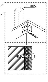
**WARNING:**INSTALLATION METHOD OF FLOATING VANITY HAS BIG RELATION WITH THE WALL STRUCTURE.
